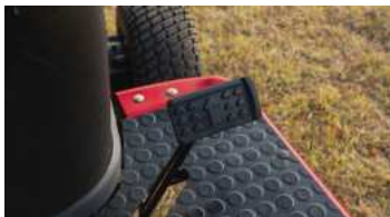
1. 2-range hydrostatic transmission (HST)
