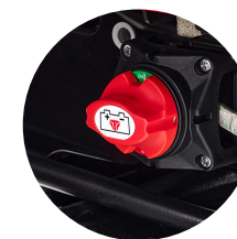
6. Battery disconnect switch
