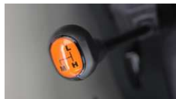
4. 8F × 8R gear transmission
