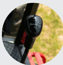
3. Joystick control for front-end loader
