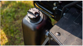
5. High-capacity fuel tank
