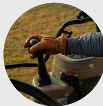
3. Joystick control for optional loader
