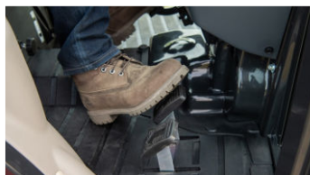
4. Highly responsive forward & reverse HST (T3035 (F36CHN))
