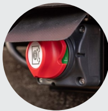
2. Battery shut-off switch
