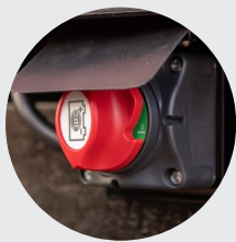
2. Battery shut-off switch
