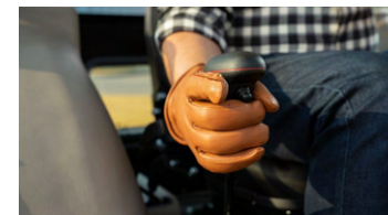
6. Joystick control for optional front-end loader
