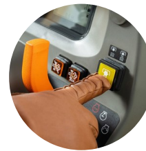
4. Independent rear PTO switch
