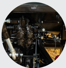
3. 4-port rear hydraulic valve
