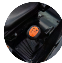
4. 3-range HST & 8F × 8R gear transmission
