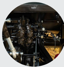
3. 4-port rear hydraulic valve
