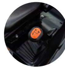
4. 3-range hydrostatic transmission
