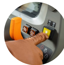
4. Independent rear PTO switch
