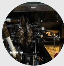
3. 2 sets of rear remote valves
