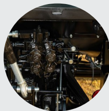
3. 2 sets of rear remote valves
