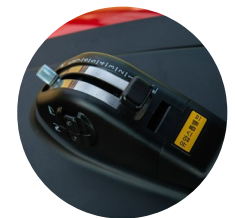
6. Electronic lift control
