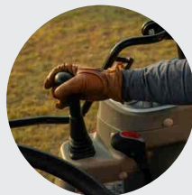
3. Joystick control for optional loader
