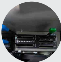
2. External lever for rear attachments
