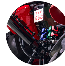
5. 8-port rear remote hydraulic valve
