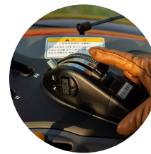
4. Electronic lift control
