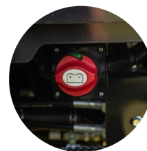
4. Battery shut-off switch
