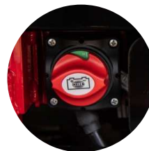
4. Battery shut-off switch
