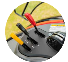
6. External hydraulic control lever
