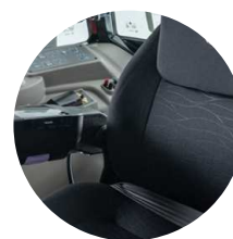
4. Adjustable suspension seat
