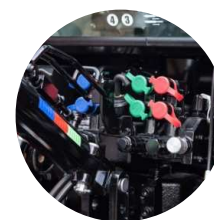
5. Rear external hydraulic ports (hydraulic top link)
