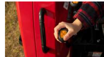
6. Joystick control for front-end loader
