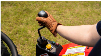
6. Joystick control for front-end loader
