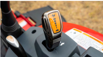
1. 2-range hydrostatic transmission (HST)
