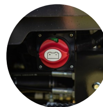
4. Battery shut-off switch
