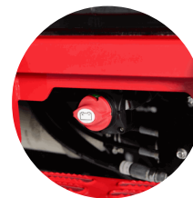
4. Battery shut-off switch
