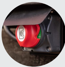
2. Battery shut-off switch
