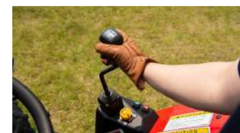
6. Joystick control for front-end loader
