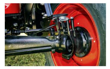
The front axle automatically disengages when the steering angle exceeds 20 degrees. At highways speeds above 10 MPH it also disengages. The push-pull dual action steering cylinder ensures precise turns, eliminating the need for a drag link.
