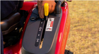
1. PTO lever for mid and rear rpm
