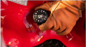
6. Dial adjustment for mower height
