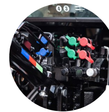
5. Rear external hydraulic ports (hydraulic top link)
