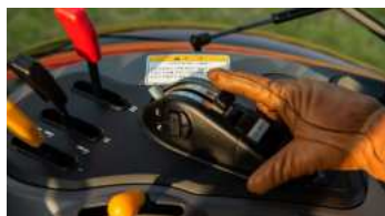
4. Electronic lift control
