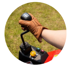
6. Joystick control for front-end loader
