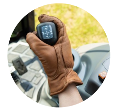
6. Joystick control for front-end loader
