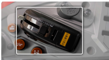
2. Electronic lift control
