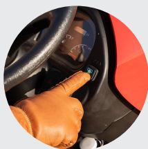
2. PTO on/off switch
