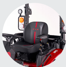
1. Mechanical suspension seat
