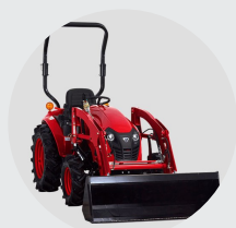
1. Optional loader with high lift capacity
