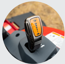
1. 2-range hydrostatic transmission (HST)
