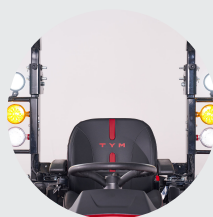
2. Integrated work signal lighting
