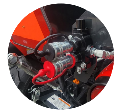
6. 2 port rear hydraulic control (optional)
