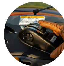
4. Electronic lift control
