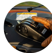
4. Electronic lift control
