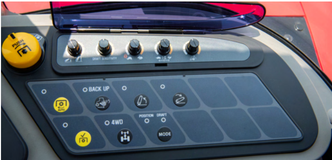
Electronic hydraulic control system with BOSCH
