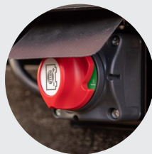
2. Battery shut-off switch
