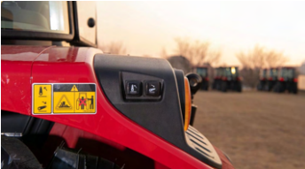
6. External hitch control buttons
