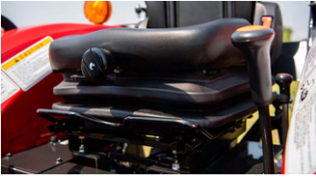
2. Comfortable suspension seat
