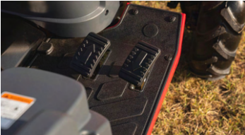
2. 2-range hydrostatic transmission (HST)
