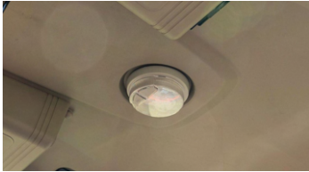
4. LED interior lighting
