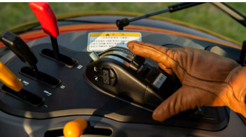
4. Electronic lift control
