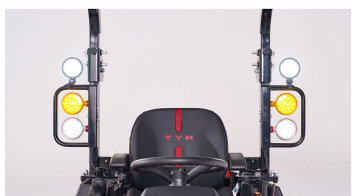
2. Integrated work signal lighting
