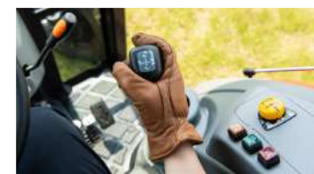
6. Joystick control for front-end loader
