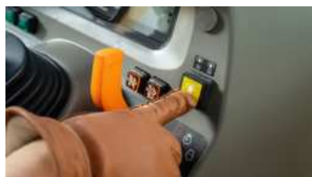
4. Independent rear PTO switch
