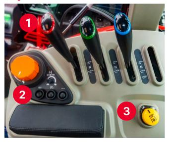
These levers simplify tasks like gear shifting and implement control, ensuring efficiency and ease of operation.
