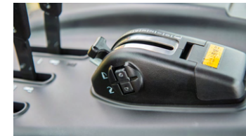
5. Electronic lift control
