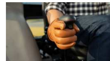
6. Joystick control for front-end loader
