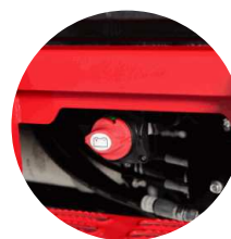
4. Battery shut-off switch
