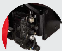
3. 6-port front external hydraulic system
