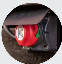
2. Battery shut-off switch
