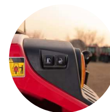
6. External hitch control buttons
