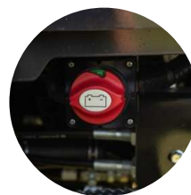
4. Battery shut-off switch
