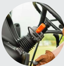
2. Hydraulic tilt / telescoping power steering
