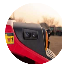
6. External hitch control buttons
