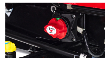
6. Battery disconnect switch
